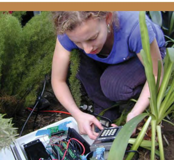
To measure flow through the xylem of the olive tree in the Lyman Conservatory, ecohydrology students set up a sap flux sensor.
